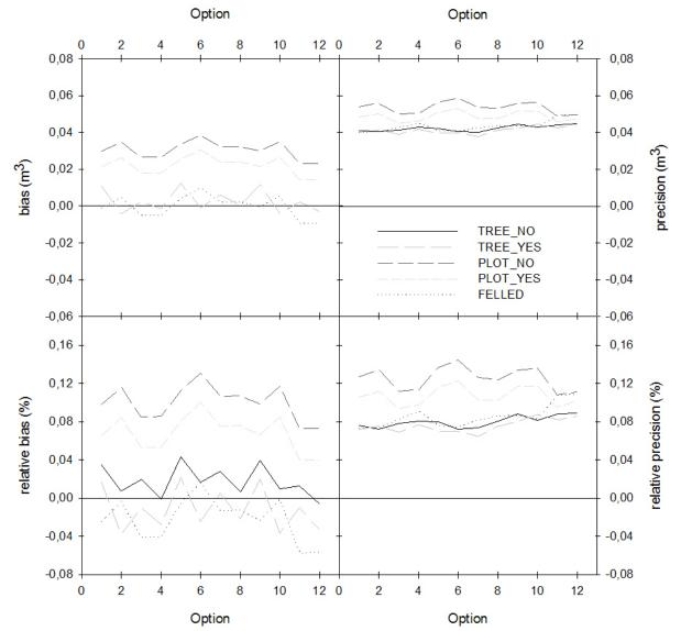
Figure 3: Representation of bias (up - left), precision (up - right), relative bias (down - left) and relative precision (down - right) through different METHOD x OPTION combinations assuming "true" volume as the one calculated with Smalian's formula
