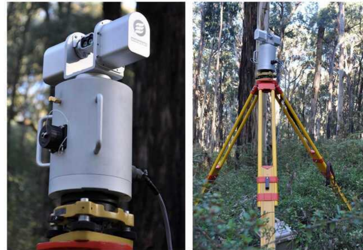
Figure 1 – LEAF instrument during operation in Eucalypt forest, Australia.
